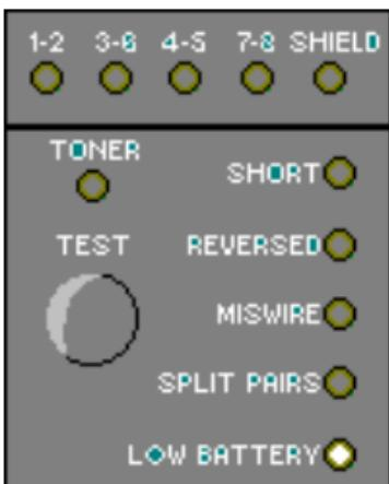
The Battery LED will light up when **MICRoMAPPER** detects a low battery condition. Using **MICRoMAPPER** with a low battery may effect the test accuracy. If **MICRoMAPPER** is stored for more than one month, the battery should be removed.
