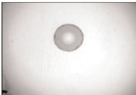
Figure 4: Good/clean fiber endface
